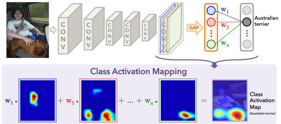
Figure 2. Class Activation Mapping: the predicted class score is mapped back to the previous convolutional layer to generate the class activation maps (CAMs). The CAM highlights the class-specific discriminative regions.
